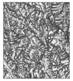
Fig. 4. Microstructure of as cast Al-4.5wt% Cu alloy.
