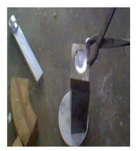
Fig. 3. Cast Iron mould used for casting Al-4.5wt% Cu alloy.
