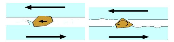
Fig. 2. Mechanism of material removal in abrasive wear.
